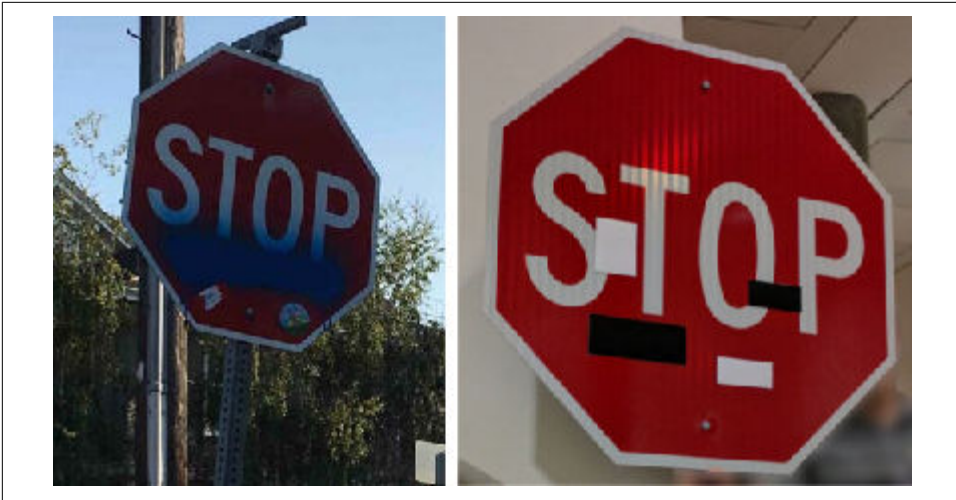
Figure 8-5. Physical perturbation applied to a stop sign (image from Eykholt et al. 2018)
