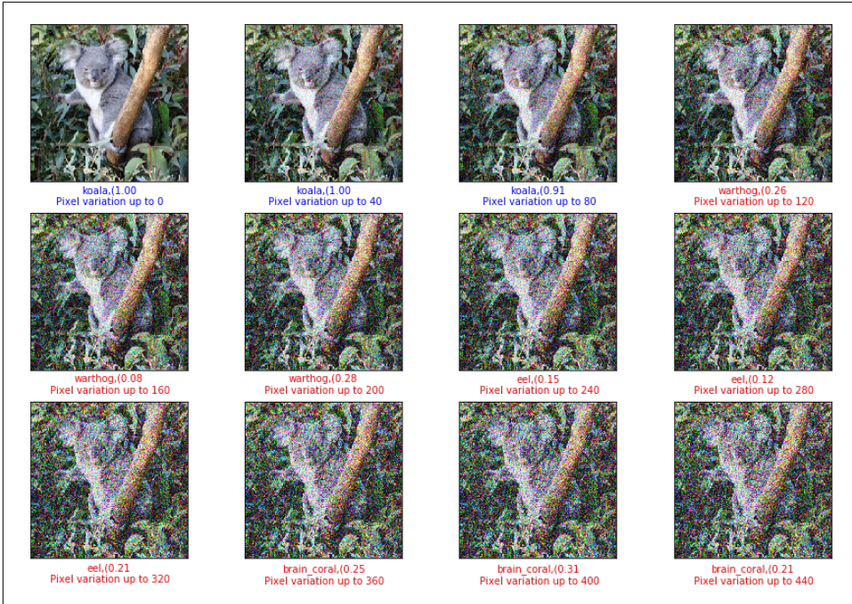
Figure 6-1. Resulting ResNet50 predictions for an image with random variation added; maximum amount of perturbation per pixel is shown for each iteration.
